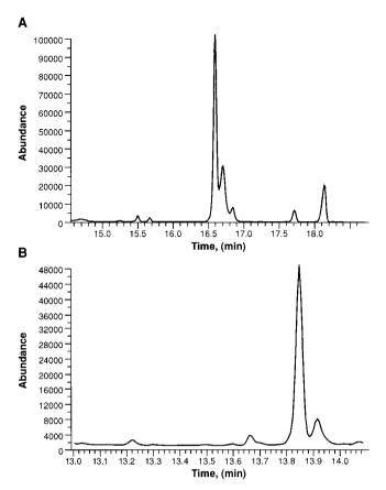
**FIG. 3.** Chromatograms of the silanized derivatives of oleamide. The m/z 338 fragments of 100 fg of N-tert-butyldimethylsilyl oleamide (A) and 100 fg of N-trimethylsilyl oleamide (B) were monitored in selected ion mode.
