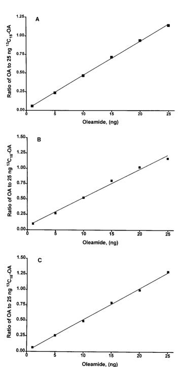
**FIG. 4.** Calibration curves for oleamide derivatives. Oleamide levels were determined by monitoring the 136/145 m/z fragment of oleonitrile (A) and the 338/356 m/z fragments of either N-trimethylsilyl-oleamide (B) or N-tert-butyldimethylsilyl oleamide (C). The ratio of the amount of oleamide to 25 ng of the internal standard,  $^{13}\mathrm{C}_{18}$ -oleamide, was plotted against the known concentration of oleamide added, and a line was fitted through the points by linear regression.
