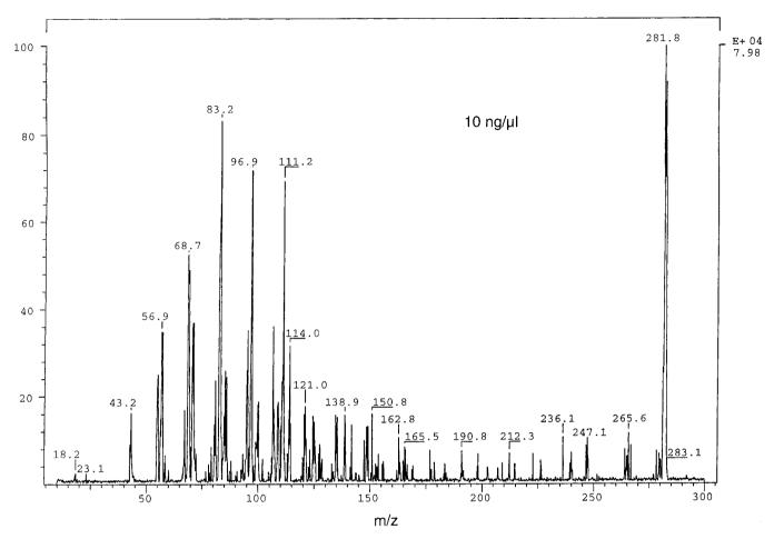
**FIG. 1.** MS/MS spectrum of  $(M + H)^+$  from 10 ng of oleamide.
